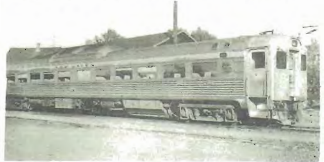
NEW SELF-PROPELLED "SHORELINER" RAIL DIESEL CAR, all stainless steel and air-conditioned, the type to be operated by The New Haven Railroad between WORCESTER and NEW LONDON.
